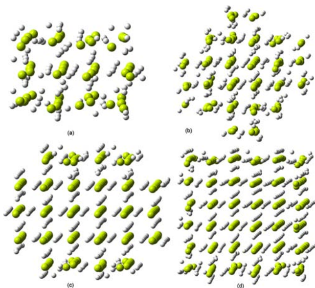
Figure 6. Optimized structures of “crystalline” (\text{MgH}_2)_N nanocrystals for N = 48 (a), 120 (b), 169 (c), and 216 (d).
